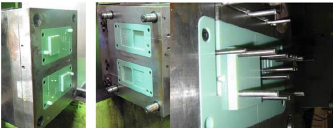
A core/cavity mold set showing a central injection point and channelling to regions where 5 different parts are formed in one cycle
