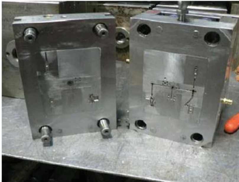
A core/cavity mold set showing a central injection point and channelling to regions where 5 different parts are formed in one cycle
